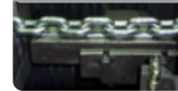
The chain is precisely sized and loaded with manufacturing proof force.
